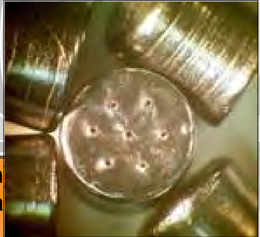
Illustration of a propellant grain cross section
